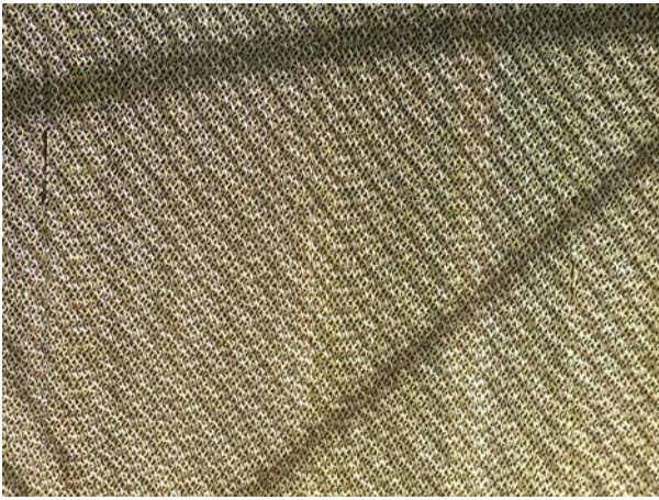
Cardboard evaporator, reinforced by \text{CaCO}_3 bio-mineralisation from seawater, and polythene tube heat exchanger.
