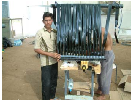
Assembly on site of the 'Watermaker' all plastic condenser.
